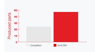
Benchmark test for M8 tap drills with 15 m/min in C45 steel carried out by a large tool manufacturer
