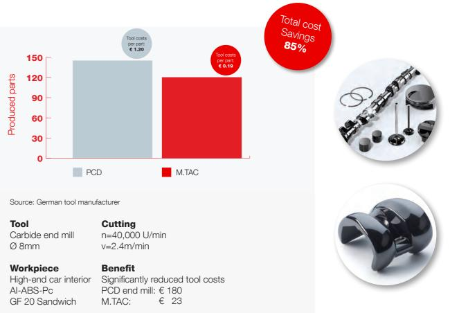
such as machining aluminium alloys, non-ferrous metals and composites like FRPs and CFRPs. Hydrogenfree tetrahedral amorphous carbon (ta-C) coatings offer exceptional performance in high-temperature environments and with extremely high hardnesses in particular.
